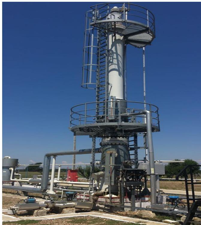
**Figure 7: Absorption column**
