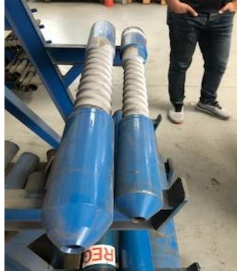
The spear is a versatile tool. It can be run in the string above an internal cutting tool or in combination with other tools, saving a trip into the hole. Milling tools may be run below the spear to open up the pipe so the spear can enter and catch.
