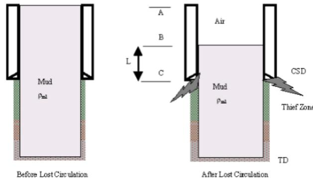
Figure 2. Mud Column High due to lost circulation
