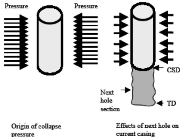
Figure 1. Collapse pressure
