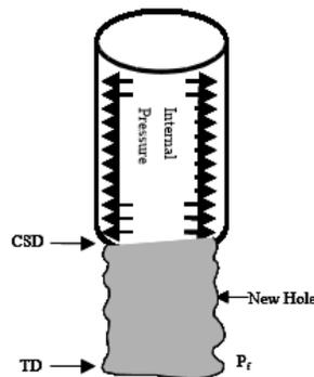
Figure 3. Burst Pressure inside the casing.
