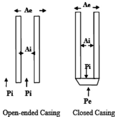
*Figure 5. Buoyancy Force.*
