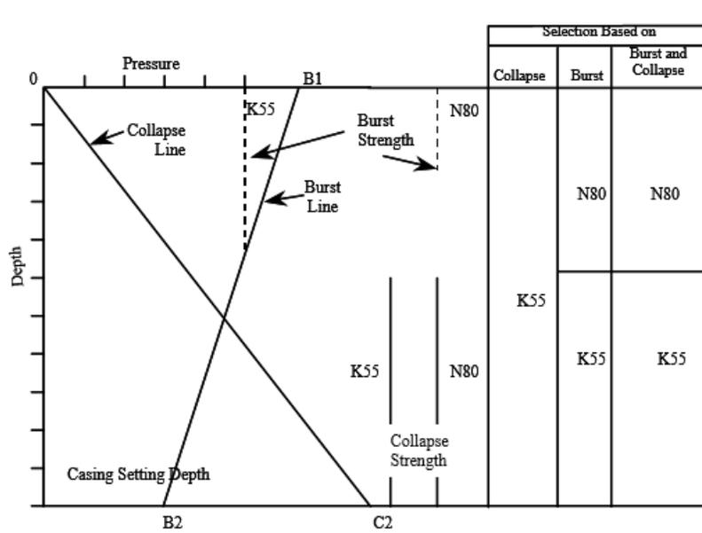
Figure 5. Selection based on Burst and Collapse.
