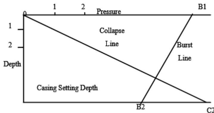
Figure 4. Collapse and Burst Lines.
